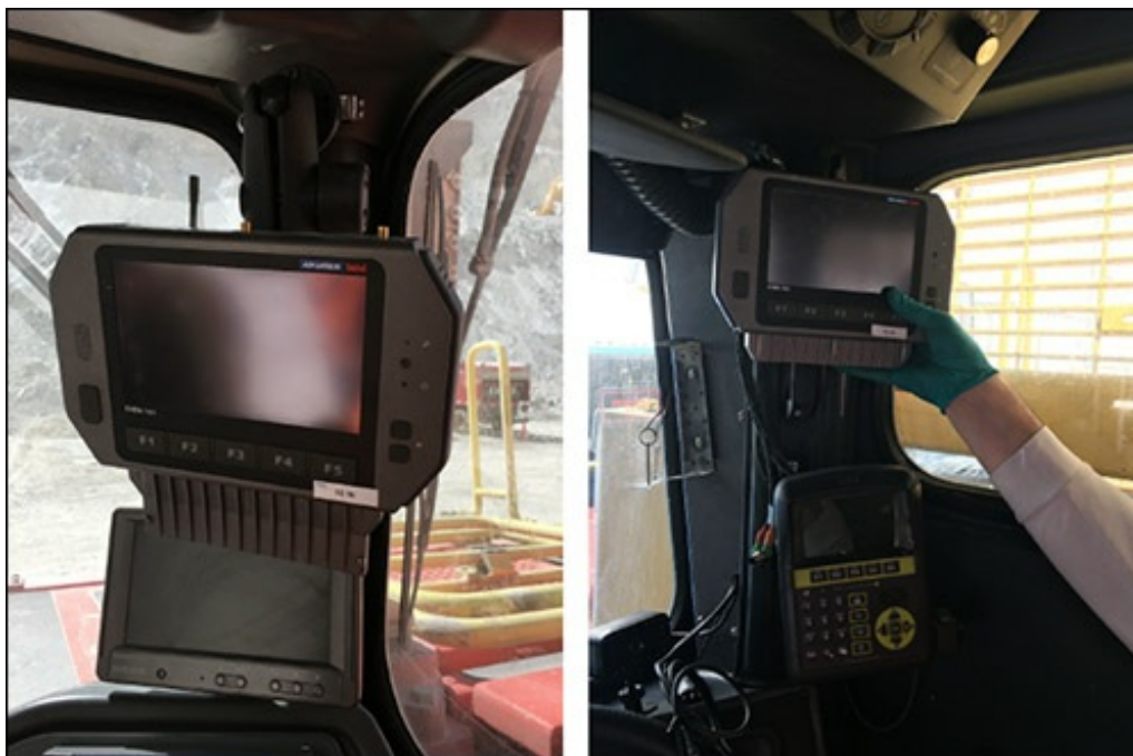
The on-board computer can access an operator's tasks for the day, which it displays on his or her screen.
